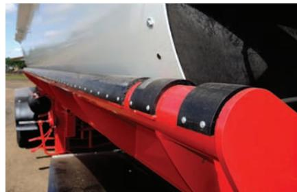
▶ High density wear resistant pads support the body along its full length as it flexes and tips. These pads are easily serviceable items when required
