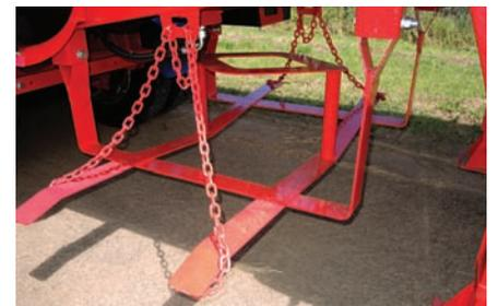
▶ A heavy duty twin tyre carrier is standard
