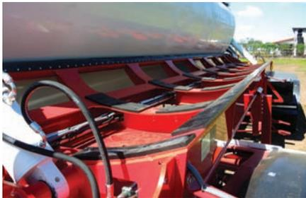
▶ HDPE pads between the tipper bowl and chassis reduce wear and improve load spreading across the chassis providing protection against impact loads
